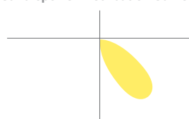
WALL WASH Candlepower Distribution Curve
